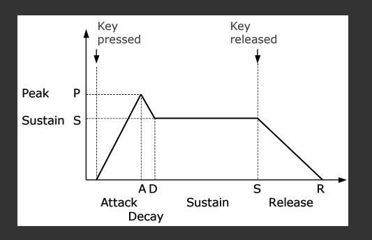
EG – envelope generator in VCA modifies changes of the signal loudness in time. The ADSR envelope consists of four sections that change linearly or exponentially.
