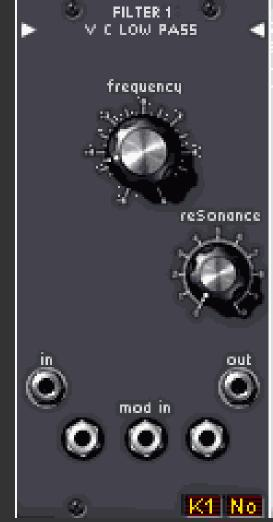
*Key follow* allows controlling the module parameters with a musical keyboard. The effect depends on the key number. If we set a fixed cut-off frequency in VCF, e.g. 2.6 kHz in a low-pass filter, then:
