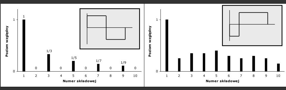
For fill rate 1:1, only odd numbered peaks are present. Changing the fill rate from 1:1 increases level of even peaks and decreases level of odd peaks.
