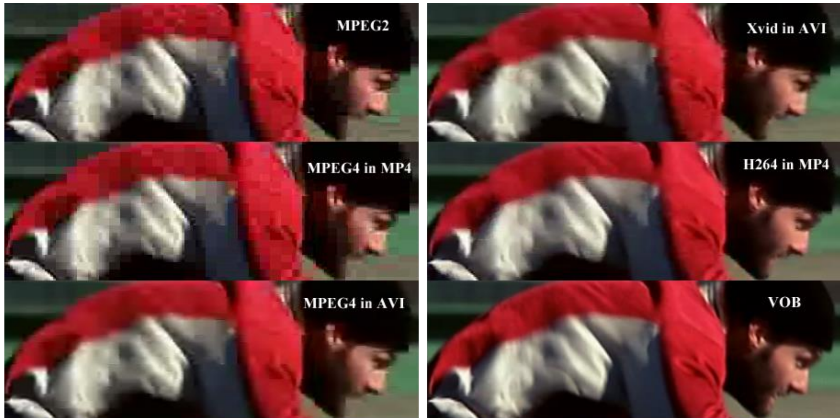
Figure 1: a small segment of a frame viewed at 100%, showing blockiness at 1000 kbps. Each macro block is 8x8 pixels. The frame is of a fast moving bike rider and the result for WMV-8 matches that for MPEG4 in MP4.
